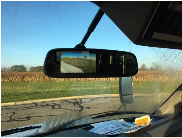
Backup Camera and Monitor Installed
